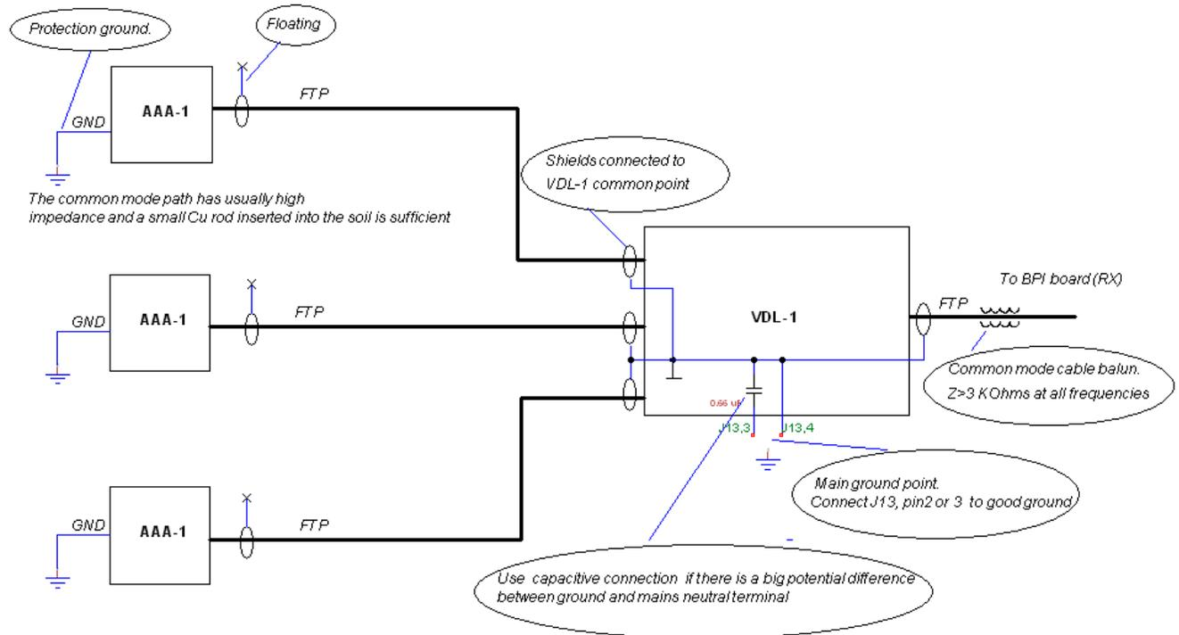
Fig.1 Ground connections and baluns of different parts of the phased array system with VDL-1 device.
