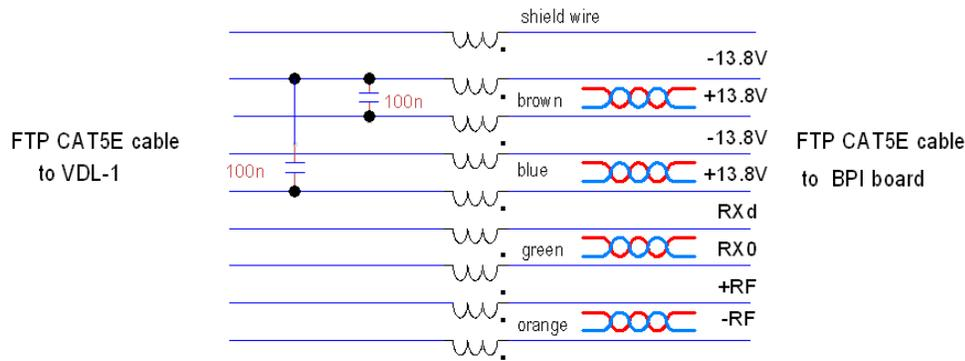
Fig.2 FTP balun schematics
