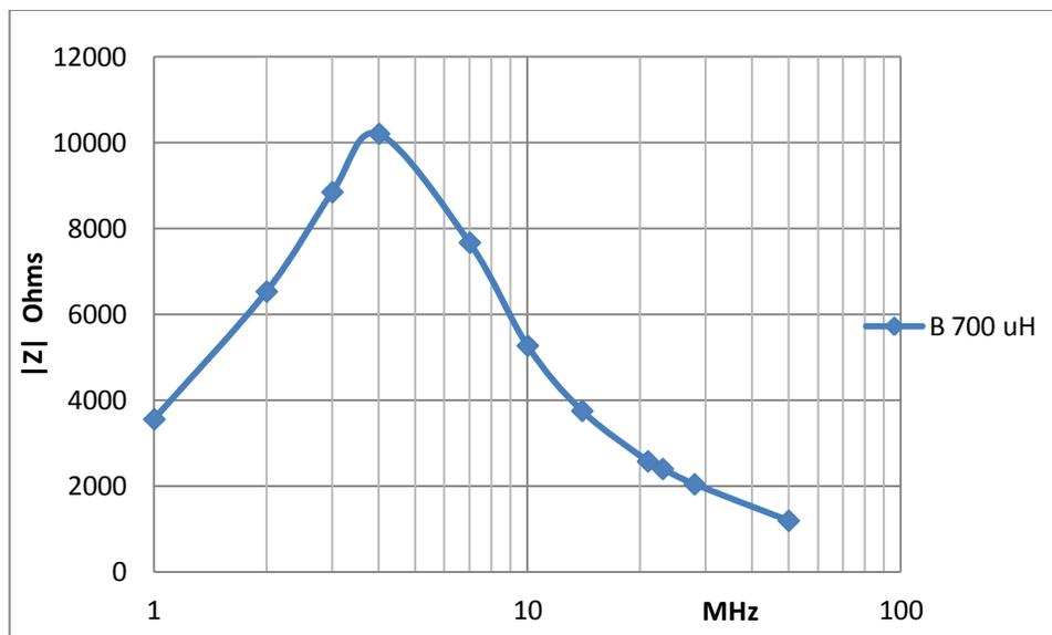
Fig.4 Impedance as a function of frequency for RF balun shown on Fig.4. This balun is very good for low bands and has acceptable impedance at 30 MHz.
