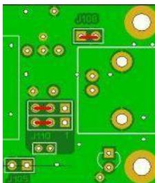
Fig.4 Limiter #1 limits to 4.2 V pp . J108 =ON, J110a 2-3 = ON, J110b 2-3 = ON
