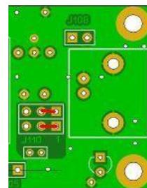
Fig.5 Limiter #2 limits to 2 V pp and 3.6 dB attenuation. J110a 1-2 = ON, J110b 1-2 = ON.
