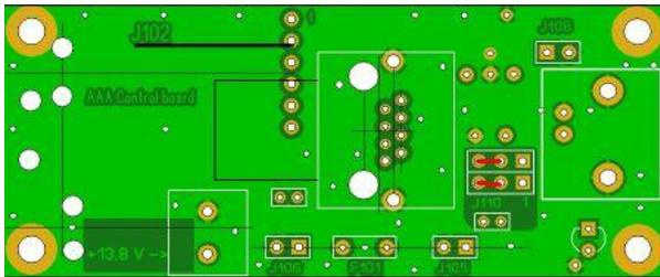
Fig.3 Normal position, no limiters J110a 2-3 = ON, J110b 2-3 = ON.
