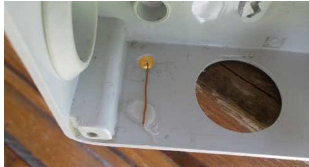
Fig.15, 16 Drainage tube is placed at the bottom side of the box. A plastic tube with external diameter 5 mm and internal diameter is 3 mm is used for this purpose. A thin wire (0.4 mm diam.) is inserted into it to reduce the effects of the water surface tension. Thus it is possible to remove also the condensed water due to very fast changes of the temperature. The drainage tube and the wire are fixed with hot glue gun. The tube can be choked if not needed.
