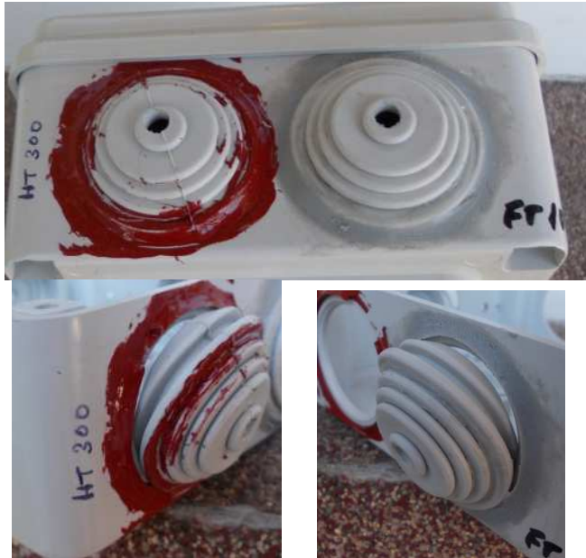
Fig.2, 3, 4 High temperature red silicone B and grey polymer sealant D (sealed and un-mounted).
