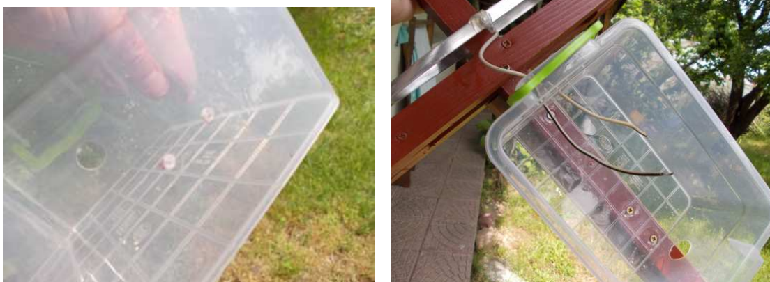
Fig.25 Several holes must be drilled in the box – for antenna terminals with 0.9 of diameter of the antenna leads. The antenna leads must pass with difficulty through these holes. Also one hole with 20 mm diameter for the FTP cable. The RJ45 plug and the rubber cap must pass freely through the hole. Another two holes (5 mm diameter) must be drilled at the lowest part of the box for water drainage.
