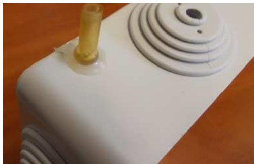
Fig.16 There is no need to seal the lower cap where the FTP cable is passing through. One small hole can be punched into the rubber cap next to the cable hole for a water drainage.
