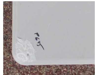
Fig.20 The holes on the cover of the box can be sealed with the same sealants. Do not fill the hole but just make a surface layer. This layer will be removed easily when the box must be opened.
