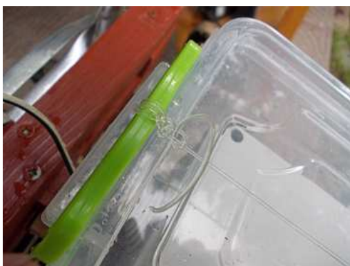
Fig.31 The cover of the protection box is secured with nylon fishing cord.
