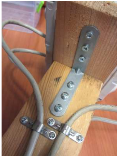
Fig.39 The plank is fixed to the stake by means of two universal clamps. Another clamps are used to fix the FTP cables.
