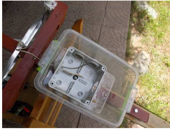
Fig.28 The AAA-1 box is mounted into protection box. It is fixed with one screw at the center of the box with rubber gasket. There is a drainage tube in the ABS box for water condense drain.
