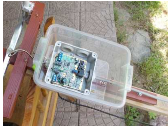
Fig.30 FTP cable and lower dipole arm (the black wire) are mounted.
