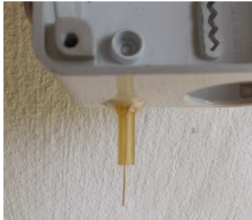
Fig.15, 16 Drainage tube is placed at the bottom side of the box. A plastic tube with external diameter 5 mm and internal diameter is 3 mm is used for this purpose. A thin wire (0.4 mm diam.) is inserted into it to reduce the effects of the water surface tension. Thus it is possible to remove also the condensed water due to very fast changes of the temperature. The drainage tube and the wire are fixed with hot glue gun. The tube can be choked if not needed.
