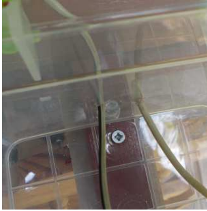
Fig.27 The antenna leads
