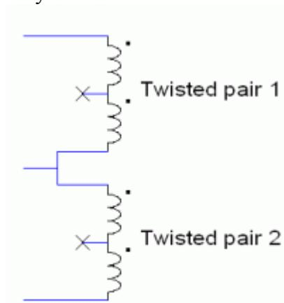
**Fig.4** A balun with reduced parasitic capacitance. The dots mark the beginning of each winding.
