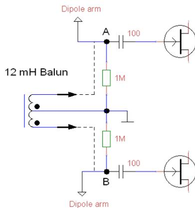
**Fig.2** The input balun ensures equal voltages referred to the amplifier common point irrespective of capacitive imbalance of dipole arms.
