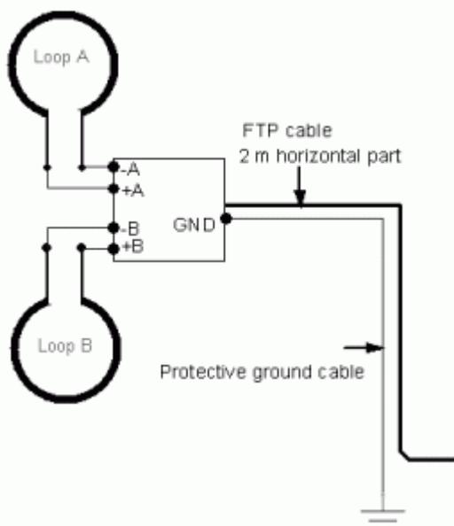
**Fig.1** Loops are used as vertical dipole arms. To improve the symmetry, the FTP and protection ground cables should run horizontally at least 1 - 2 m from the loops. Also exchanging terminals of Loop A and B might give better symmetry. These measures refers only for dipole mode and do not influence the loop modes.
