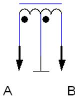
**Fig. 3** The inductance is measured between A – B points
