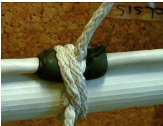
**Fig. 4.13** Old fashioned marine style fix with double constrictor knot. Use thin polyester rope which is UV resistant and will last for many years. Again a self-amalgamic tape is used as a protector.
